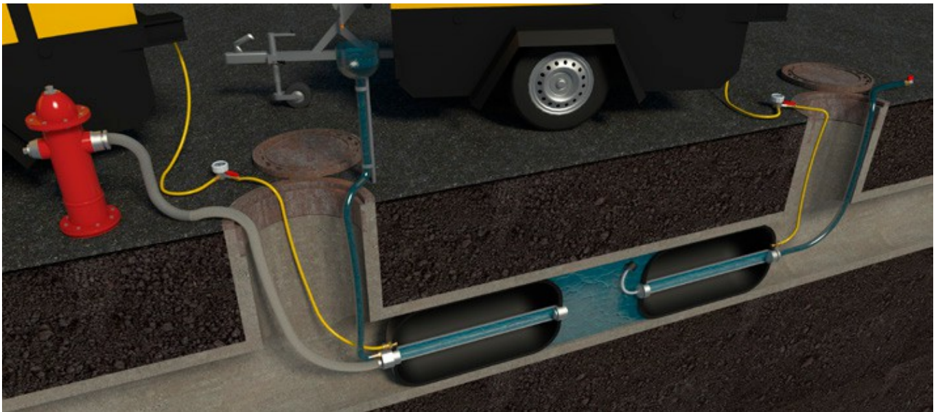
Figure 35: Water leak test of pipelines
