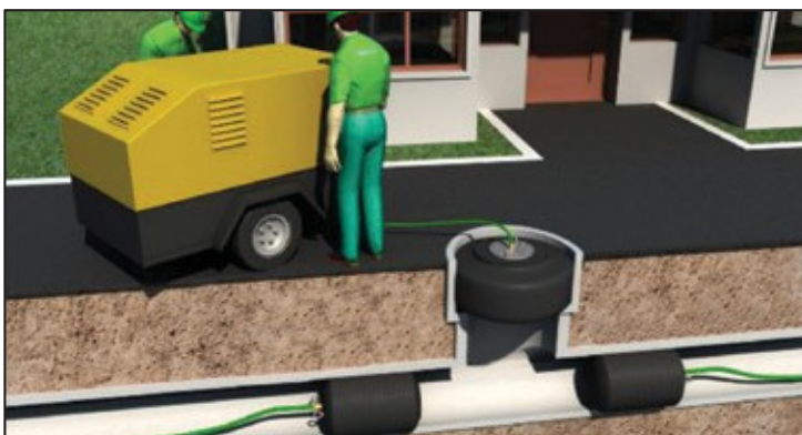
Figure 36: Gully leak test
