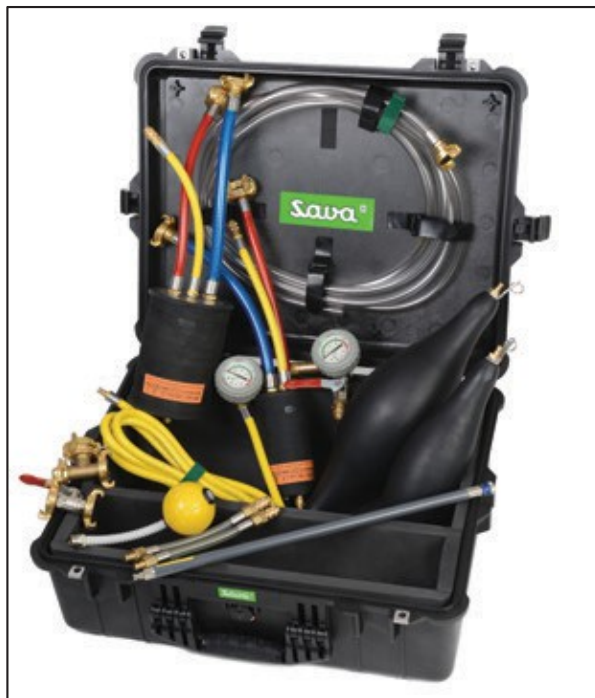
Figure 37: House connection leak test
